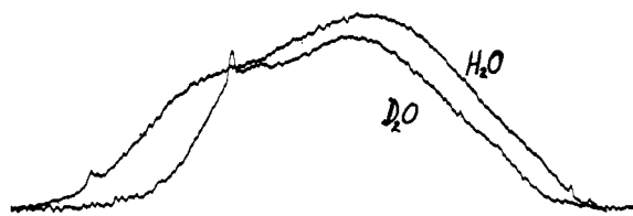
Fig. 5.—Main bands of H 2 O and D 2 O superimposed for comparison of shapes.
